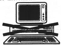
The top of the VDT should be slightly below a horizontal eye level. [I would professionally recommend 30° below eye level - similar to the aspect of a book when read. In the case of IBM machines, this means NOT stacking your monitor on the CPU. MF]
